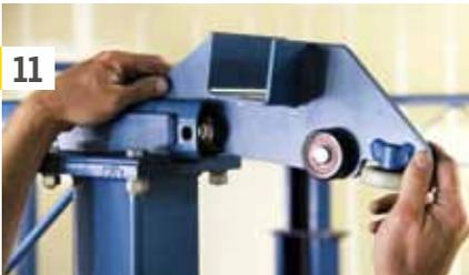
An end truck was threaded onto each end of the runways' tracks. Each end truck has four vertical wheels and two horizontal wheels to allow it to move freely. The bridges will be secured to these end trucks. There is no need to grease the tracks, in fact Loughlin recommends against it. Just take an air hose and periodically blow the tracks clean.
