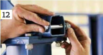
A bolt was threaded across the end of each runway's tracks to keep the end trucks from sliding out and falling onto the ground. Take care not to pinch the tracks by over-tightening the stopper bolts.
