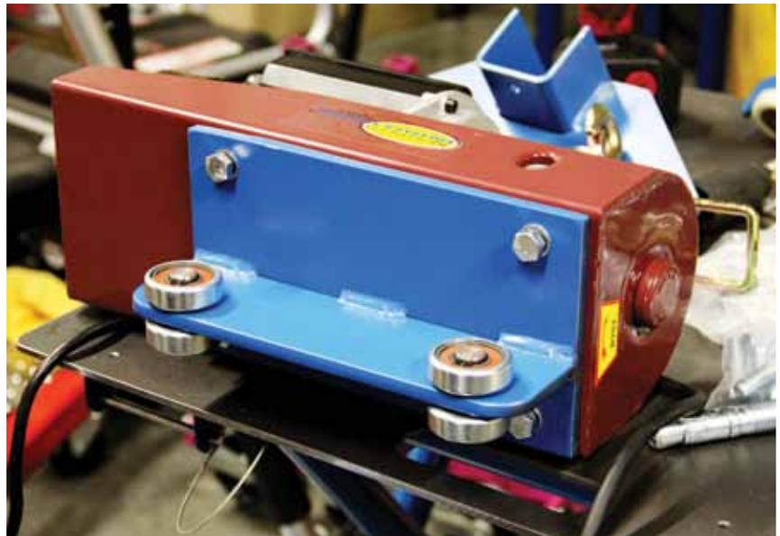
With the structure almost complete, we turned our attention to our hoists and bridges. To prepare the hoists to mount on the bridges, Kunda bolted a trolley onto the top of each one, which allows them to be threaded onto the bridge.
