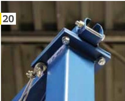
To hold up the extension cord, we removed two of the bolts on the inside of the columns on the electric side and installed a cable spanning the length of the runway before retightening the bolts.
