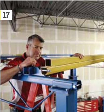
After turning the bridge right-side-up onto the forks of our forklift, we lifted the bridges lengthwise to place them onto the end trucks of either runway. We realize not every shop has a forklift and if yours doesn't go ahead and put the bridge up first and then follow up by putting the trolley once the bridge is in place.
