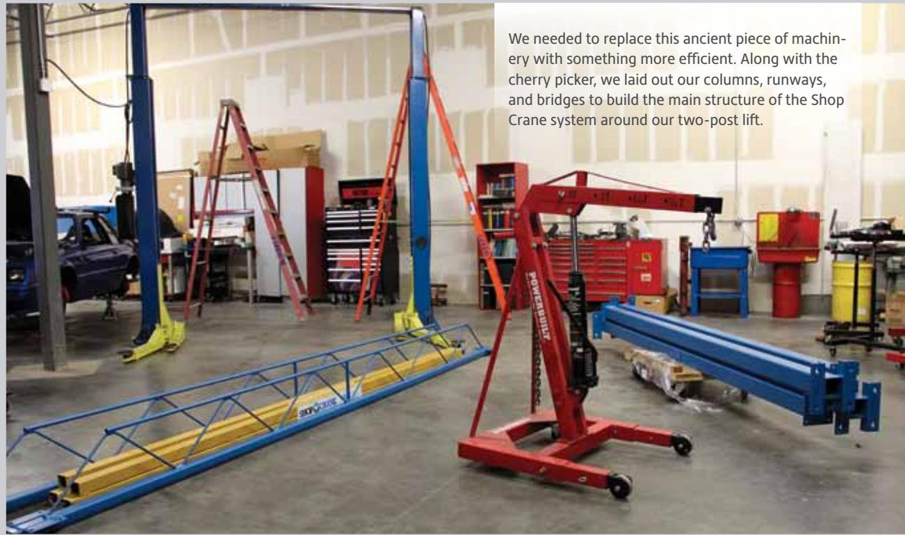
We needed to replace this ancient piece of machinery with something more efficient. Along with the cherry picker, we laid out our columns, runways, and bridges to build the main structure of the Shop Crane system around our two-post lift.
