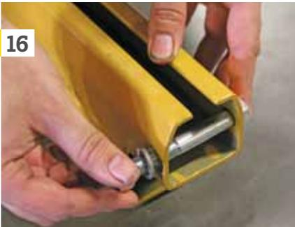
Stopper bolts were tightened onto the ends of each bridge to lock them into place atop the end trucks and ensure fit and stability once installed.
