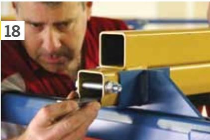
Tapped and threaded plates were slipped into the ends of each bridge and bolted down to gap the track so that the ends can't clamp. This is done just in case there is a slight misalignment in the runways, so that the end trucks will have the ability to float in and out just a little bit while the bridge runs up and down the runway.
